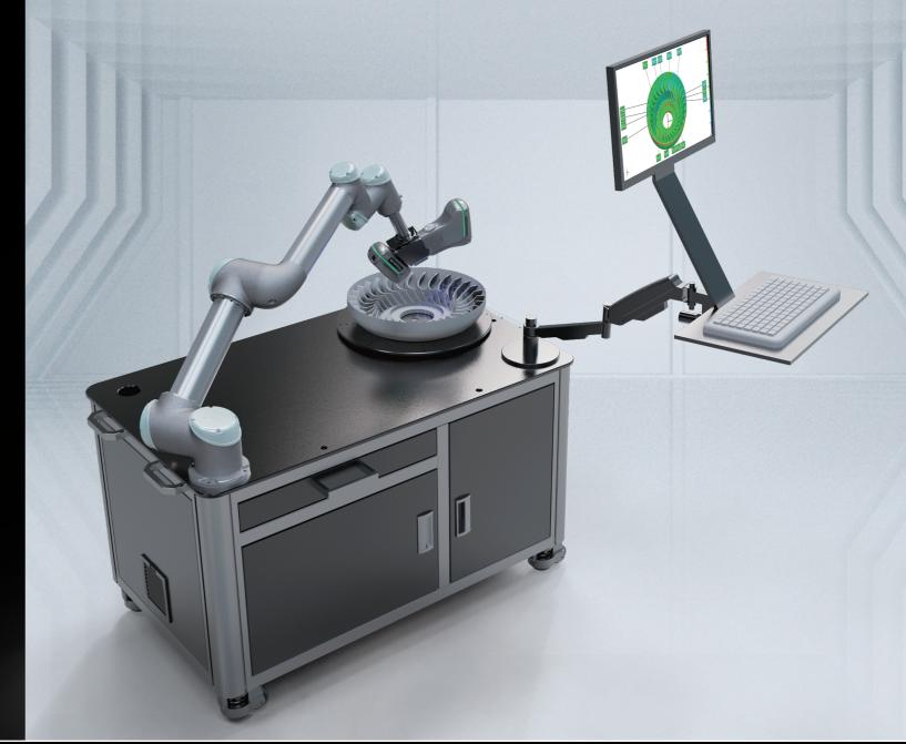
AutoScan-K series, an automatic 3D inspection system, can realize non-contact and non-destructive inspection using machine vision technology. While ensuring extra-high accuracy, it can effectively carry out online batch scanning and inspection. Featuring 24-hour constant operation, AutoScan-K 3D system helps enterprises reduce manufacturing costs, accelerate product time-to-market and increase return on investment.
